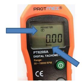
4. Place the Large Wheel in contact with the handrail and then momentarily depress the "Measure" Key. The display should indicate a handrail speed of approximately 75 feet per minute.
