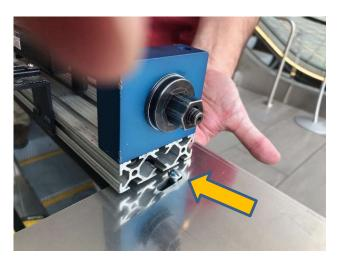
9. Fit the Gripper Assembly over the handrail, then place the red block of the Gripper Assembly onto the EsKalometer's main foot's toe and then install the tethered securing pin.
