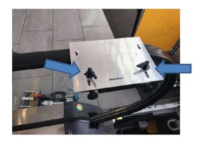
2. Loosen both Jack Screw Knobs (black knurled), located adjacent to the Black Handle, until they are fully retracted.
