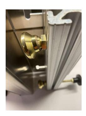
3. Grasping the Black Handle, located just below the top surface of the Balustrade Clamp, pull the clamp jaws to their fully open position.
