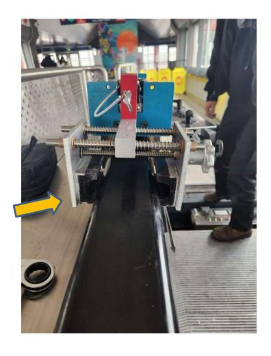
The side plates have two locating holes for the Gripper Pads. Should the Gripper Pads not align with the handrail, relocate them into the lower/upper set of holes in the side plates.
