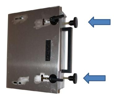
8. Slide the EsKalometer's frame onto the top of the Balustrade Clamp aligning the center tee slot with the floating restraining screws so that the centerline of the EsKalometer and the handrail are generally in-line with one another. NOTE: No adjustment of these screws is necessary.
