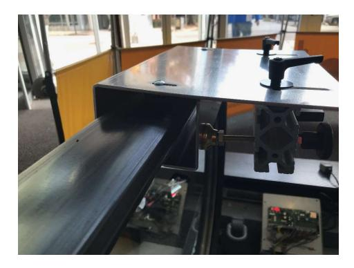
5. Push the double clamp jaws closed around the balustrade via the Black Handle until the levers slip into the top edge of the "T" slots, then tighten the Black Securing Levers.
