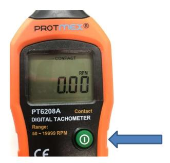
3. Depress the "MODE" Button three (3) times, the display should now read "Ft/Min" on the lowest line of the display and the PERIMETER: Box should display [6"].
