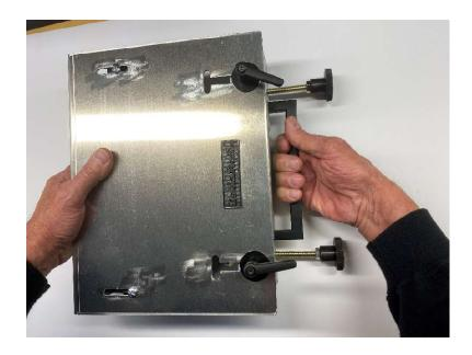
4. With the escalator STOPPED, place the EsKaRail Balustrade Clamp over the handrail and allow it to rest onto the top surface of the handrail.
