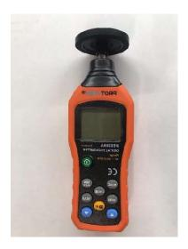
2. Depress the green button to turn the tachometer on. The primary display will read as below (RPM).
